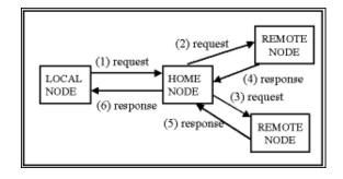
Figure 1: Nodes Involved in a Shared Memory Transaction
