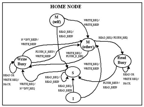
Figure 4: Home node State Transition Diagram
