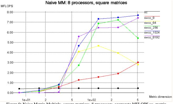
Figure 9: Naive Matrix Multiply, square matrices, 8 processors, aggregate MFLOPS vs. matrix dimension.
