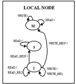
Figure 3: Local node State Transition Diagram
